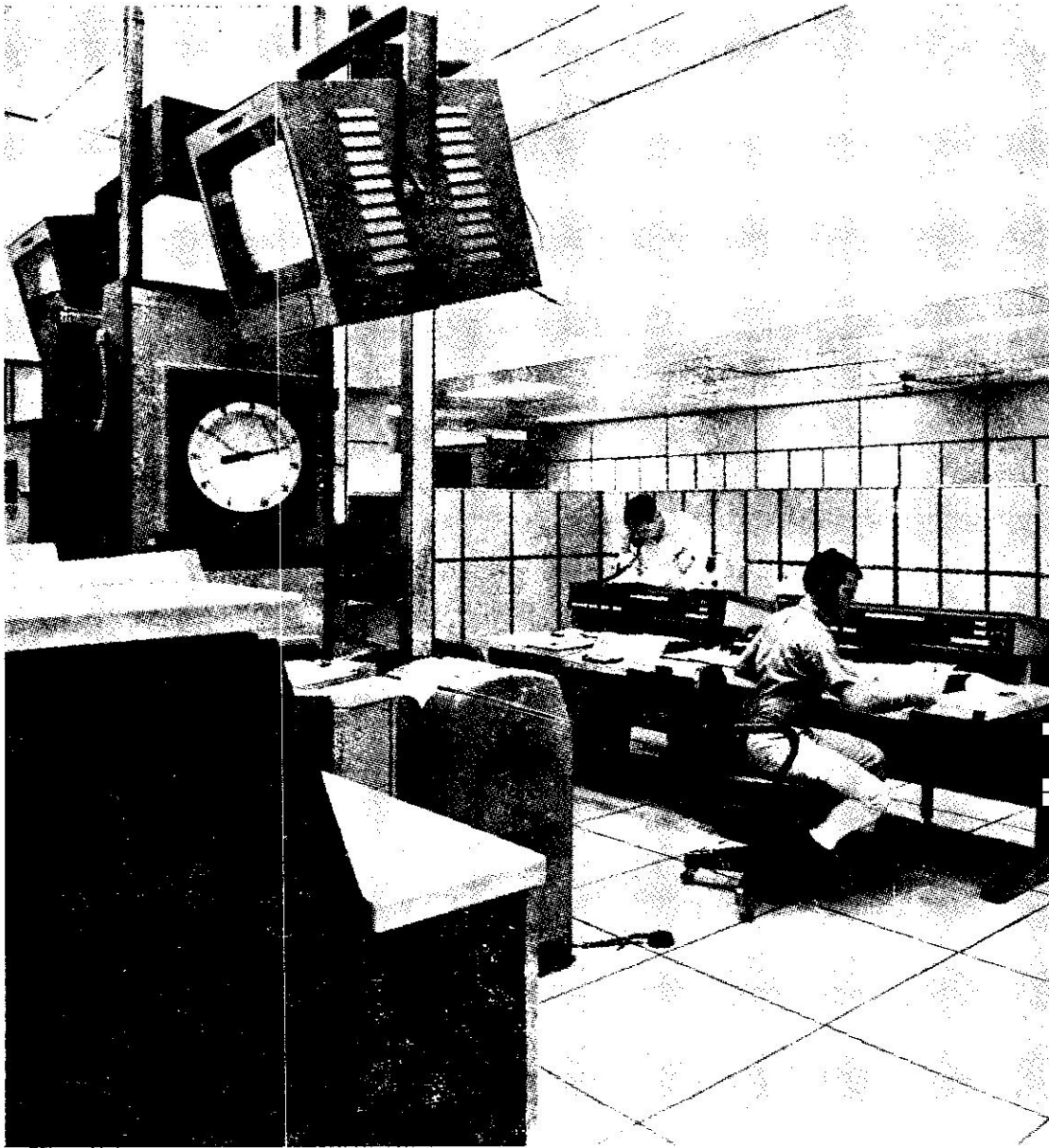
Large-scale UNIVAC 494 Real-Time Computing Systems anchor NASA's worldwide Space Flight Network communications system. Serving as communications processors, provide the speed of computer control to handle, process and route the flood of communication between Apollo spacecraft and Mission Control in Houston. These are over 15 times more than those used in the Gemini programmes.
