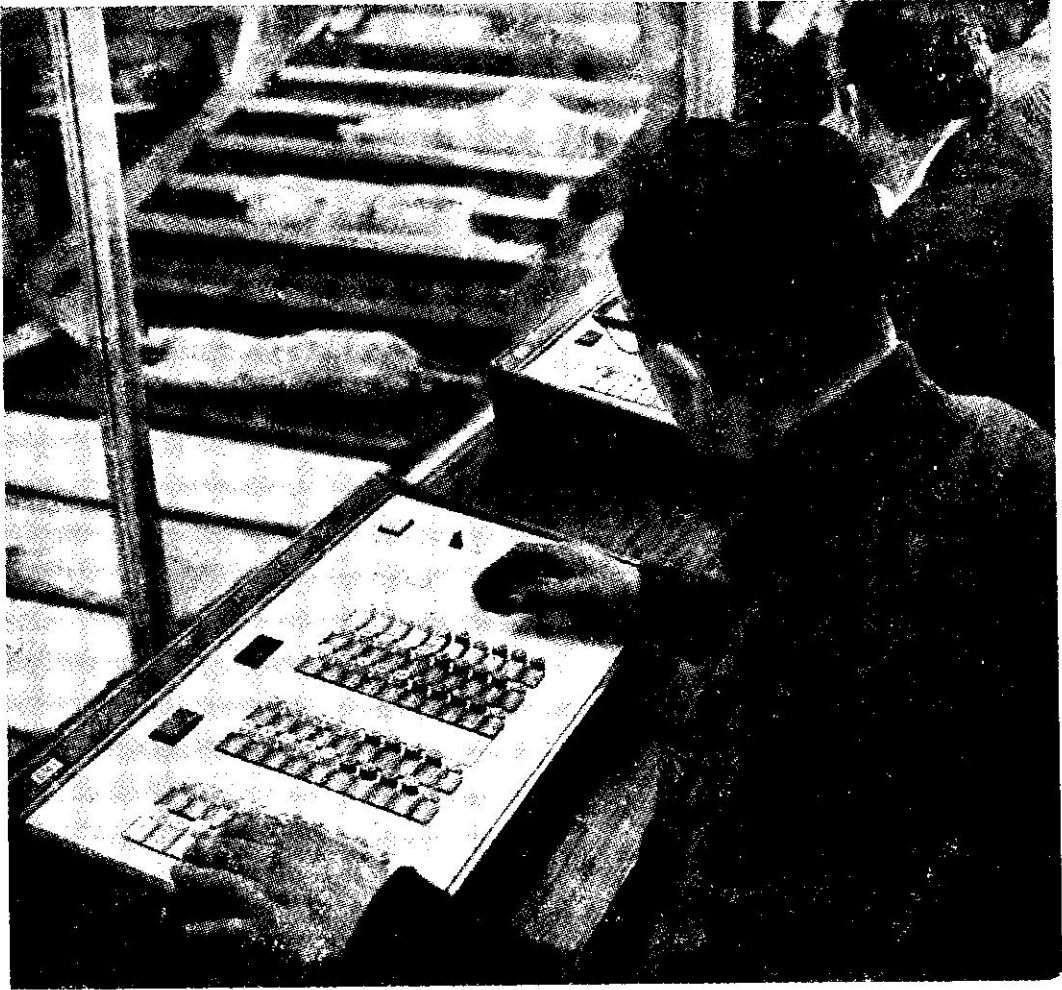
Operators, each provided with a key-board with seven columns of 10 keys, pressing keys to identify trays of meat
